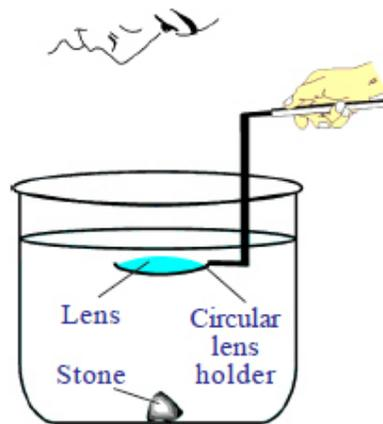
6. Set the distance between stone and lens that is equal to or less than focal length of lens.
