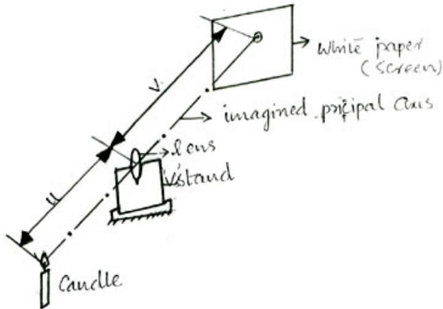
6. Now place the candle at a distance of 60cm from lens, try to get an image of candle flame on the other side on screen. Adjust the screen till you get a clear image.
