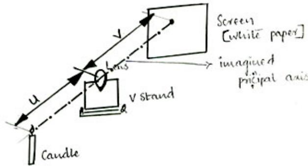
5. Measure the distance of image from the v stand of lens (image distance 'v') and also measure the distance between candle and stand of lens (object distance 'u'). Record the values in table.
