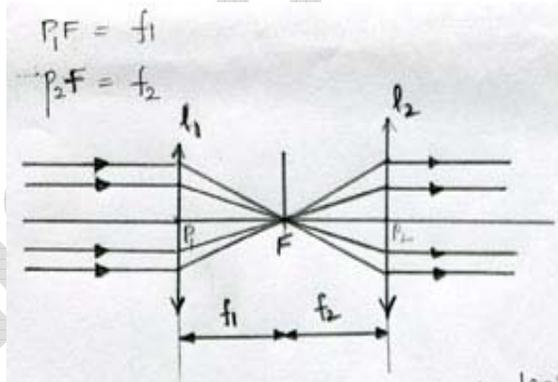
From above figure, two convergent lenses are to be placed in a path of parallel rays, so that the rays remain parallel after passing through both lenses by separating the lenses at a distance of  $f_1 + f_2$  units apart.
