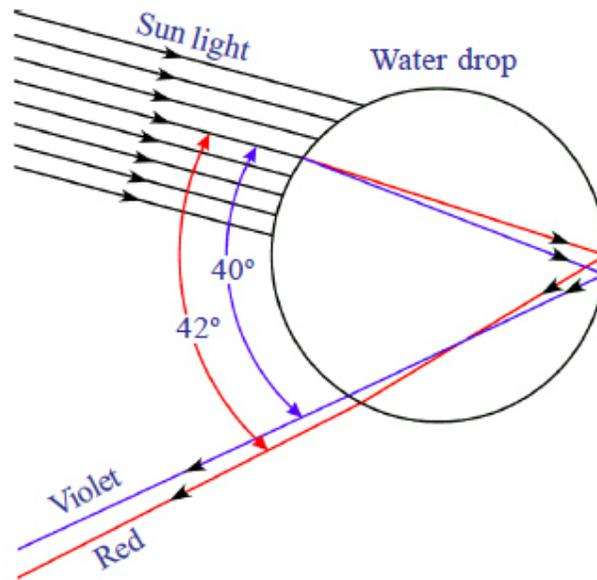
4. Arriving at the surface of the drop each colour is again refracted into air
