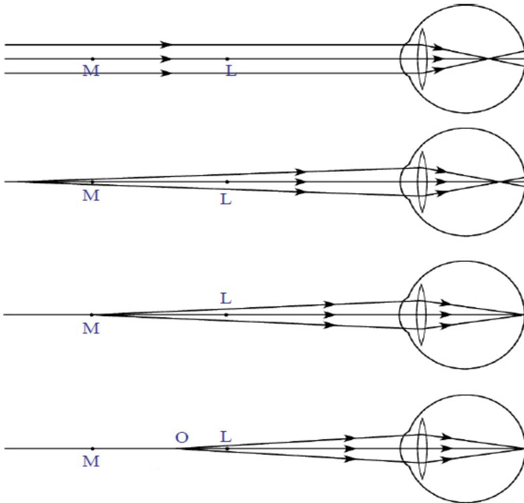
4. If we are able to bring the image of the object kept beyond far point, between far point and the point of least distance of distinct vision using a lens, this image acts as an object for the eye lens
