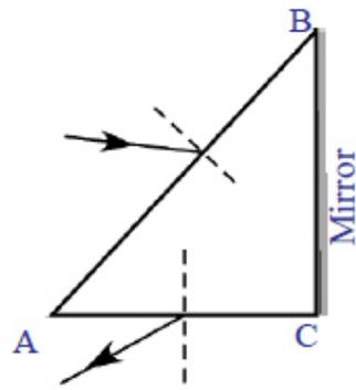
A. Here AB, AC are refracting surface and BC is reflecting surface. Incident ray enters into prism (denser medium) from air (rarer medium) so it bends towards normal.
